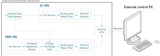
The ionization in the EI-MS takes place at 70 eV and the mass range is from 1 to 100 amu with a resolution of 1 amu. The temperature- and pressure compensated sample gas inlet guarantees correct measurements and avoids any discrimination of the gas.
